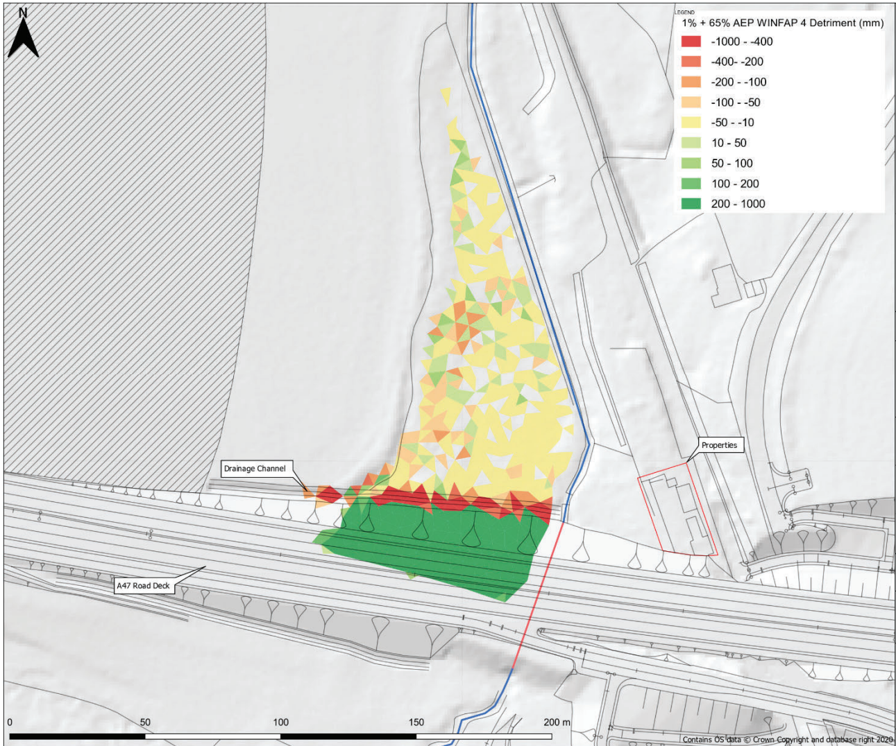
Caption 7.8 - The 1 in 100-year plus 65% climate change allowance flood depth difference map
